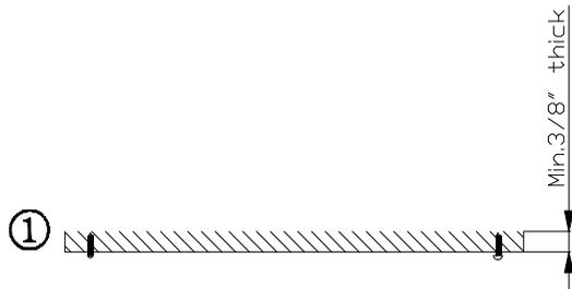
2. Install the 4 plastic anchors 46 1/2" apart and 3.189" apart, then screw into each anchor. Spacing between ceiling and cap nut should be at least 1/3".
