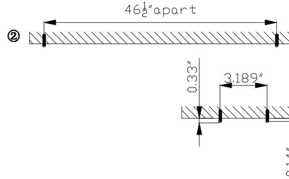
3. Lift fixture up to screws and slide to one side to secure into place. Screw size: ST4X30.
