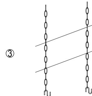
4. Install the "S" hook from one end of the chain into the end cap of the LED lamp, then crimp the hooks end with pliers. Repeat same step for the opposite side.
