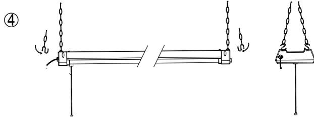
5. Install the LED lamp with chains, one end at a time onto each screw eye hook. Once installed, crimp each of the "S" hooks end with pliers. Please noted the on/off pull chain is 9.8 inches long.
