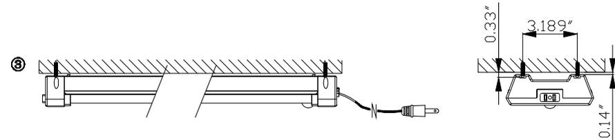
4. Plug the power supply cord into the electrical outlet.
