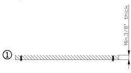
2. Install the 4 plastic anchors 46 1/2" apart and 3.189" apart, then screw into each anchor. Spacing between ceiling and cap nut should be at least 1/3".
