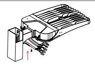
Step 2.Use tools to fix the lamp on square lamp pole, connect the wires correctly and make waterproof measures well, close the junction box and finish installation.
