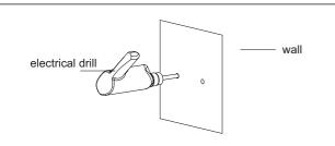
Step 1.Mark the position of the fixing holes with foold lightbracket, then drill the fixing holes.
