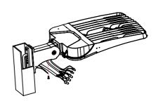
Step 2.Use tools to fix the lamp on square lamp pole, connect the wires correctly and make waterproof measures well, close the junction box and finish installation.
