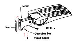
Step 1.Use tools to take screw apart and put installed iron bar away, remove fixed screw and open junction box, then pass the AC wire through it.
