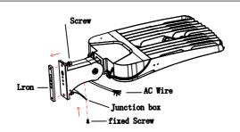
Step 1.Use tools to take screw apart and put installed iron bar away, remove fixed screw and open junction box, then pass the AC wire through it.
