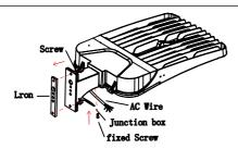
Step 1.Use tools to take screw apart and put installed iron bar away, remove fixed screw and open junction box, then pass the AC wire through it.
