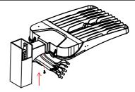
Step 2.Use tools to fix the lamp on square lamp pole, connect the wires correctly and make waterproof measures well, close the junction box and finish installation.
