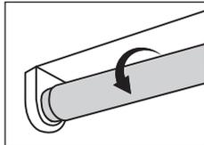
2. Remove diffuser (if provided), remove existing fluorescent lamp(s) from luminaire. Note: Verify that the fluorescent tube type is listed on the LED lamp label.
