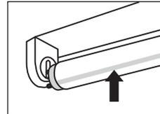
3. Install LED lamp (one for each fluorescent lamp removed, ensure pins are firmly seated in lampholders).
