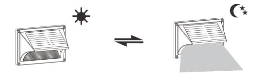
The light is automatically off in the daytime while the solar panel charges.
