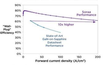
Source: Competitor data sheet, and Soraa internal data at 85°C junction temperature
