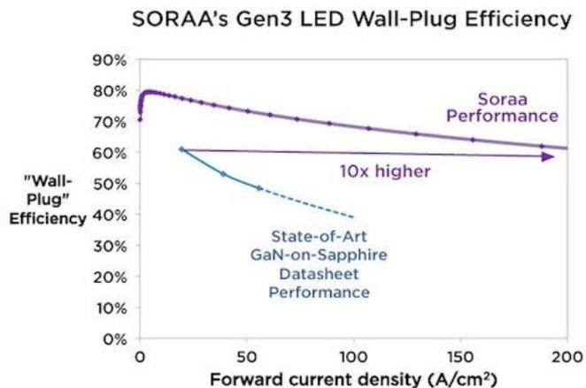
Source: Competitor data sheet, and Soraa internal data at 85°C junction temperature
