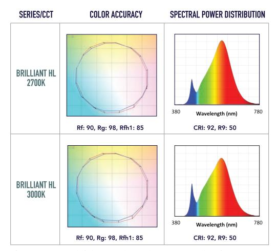
Rf: TM-30 metric measuring color fidelity (whether colors are similar to those under natural light). Rf is a more accurate version of the CRI Ra. Rf is 100 for natural light. Rg: TM-30 metric measuring color gamut (whether colors are more saturated than under natural light). Rg is 100 for natural light. Rfh1: TM-30 metric measuring color fidelity for red tones. Rfh1 is a more accurate version of the CRI R9. Rfh1 is 100 for natural light.
