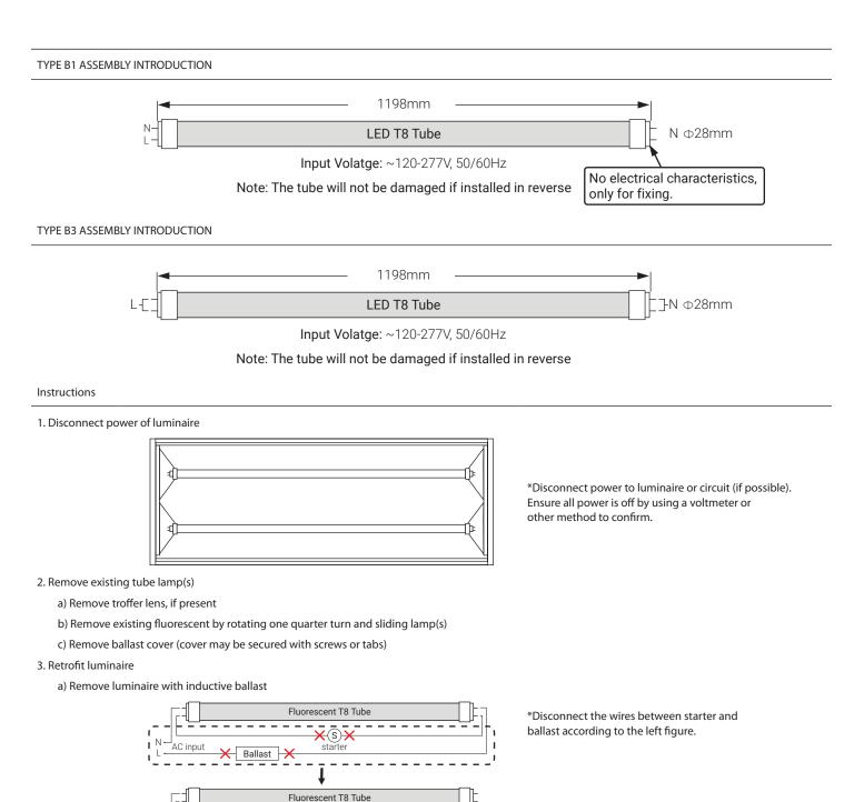
\*Connect two wires to branch circuit L and N according to the left figure.
