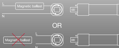
When used with a magnetic ballast, the PL H can function as a plug & play lamp and operate with the existing ballast. If the ballast is not compatible, it can be bypassed and the lamp can run directly off line voltage.
