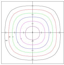
Horizontal Footcandles Scale: 1 Inch = 25 Ft. Light Loss Factor = 1.00 Lumens Per Lamp = N.A. (absolute photometry) Luminaire Lumens = 25089 Mounting Height = 25.00 Ft Maximum Calculated Value = 5.86 Fc Arrangement: Single
