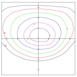
Horizontal Footcandles Scale: 1 Inch = 25 Ft. Light Loss Factor = 1.00 Lumens Per Lamp = N.A. (absolute photometry) Luminaire Lumens = 24635 Mounting Height = 25.00 Ft Maximum Calculated Value = 7.55 Fc Arrangement: Single
