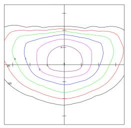
Horizontal Footcandles Scale: 1 Inch = 25 Ft. Light Loss Factor = 1.00 Lumens Per Lamp = N.A. (absolute photometry) Luminaire Lumens = 25151 Mounting Height = 25.00 Ft Maximum Calculated Value = 7.11 Fc Arrangement: Single
