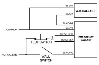
① Select proper voltage lead. Cap unused lead.
