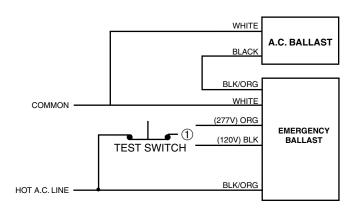
1 Select proper voltage lead. Cap unused lead.
