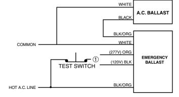
(1) Select proper voltage lead. Cap unused lead.
