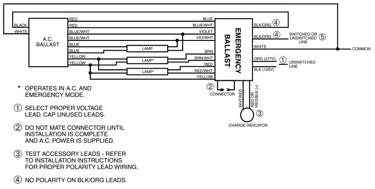
(5) SWITCHED OR UNSWITCHED LINE-REFER TO INSTALLATION MANUAL FOR HOT AND TEST SWITCH PLACEMENT.
