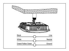
2: Connect the wires threaded from conduit and Canopy, Black wire for Line, White for Neutral, Yellow Green for Ground.
