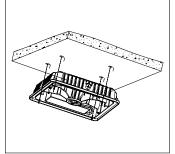
2: Cut off the wires through from 3/4" hole and plug the hole with provided Plug. Drill 4 holes on edge of fixture and fix it on the ceiling with using appropriate screws.
