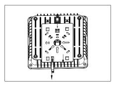
**1:** Loosen the screw on side of the light, removing the bracket from Canopy light by pulling it slightly out, just leaving the ring on bracket. ( See the Step 1 above)
