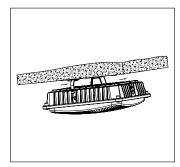
**4:** Slide the Canopy lights into bracket, and secure the screw on side of the light to prevent the light from sliding out from the bracket. Installation done.
