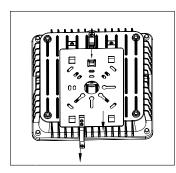
1: Loosen the screw on side of the light, removing the bracket from Canopy light by pulling it out slightly, just leaving the ring on bracket.
