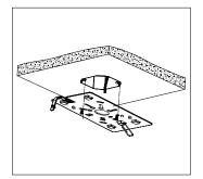
2: Fix the bracket on J-box, and put the wire through the central hole for wiring.
