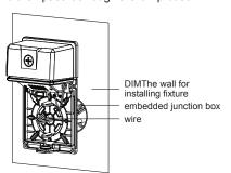
6.Lock the lamp base with the screw on the embedded terminal box.
