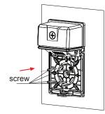
7.Connect the lamp input line, then put the connected wires into the embedded terminal box.
