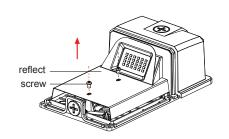
3.Put the pad on the concave side of the lamp. It aims to avoid the damage of back shell when it struck by hammer. Then hammer the plugs of the cable entry and mounting hole.
