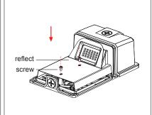
9.Use screws to tighten up the lamp, then installation completed.
