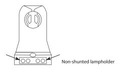
**NOTE:** If using existing non-shunted lamp holders, Installer should not disconnect lead wires from lamp holders and make new connections at terminals. Instead, cut lead wires away from lamp holders and make new connections to lead wires using approved connectors.
