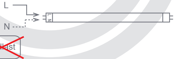
Diagram 3 – Single tube wiring
