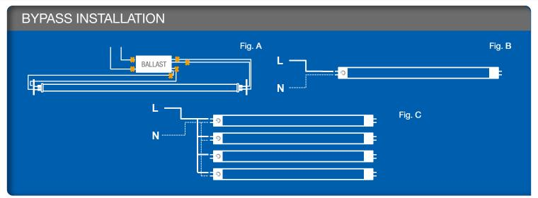
Bypass ballast by cutting all wires as in Fig. A
