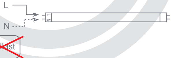
Diagram 3 – Single tube wiring
