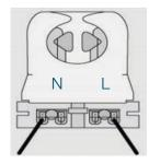
On the end cap, the pin with 'L' marking must be latched into the side of tombstone connected to the hot wire. 'N' marked pin must be latched into the side of tombstone connected to neutral wire.
