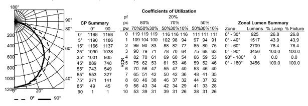
2AVL4 40L MDR LP835, 4255 delivered lumens, test no. 69071P5, tested in accordance to IESNA-LM79.
