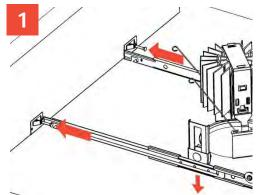
Mount to joists with flanges on channel bars resting against the bottom faces of the joists. Drive included nail into joist to secure. Move vertical adjustment to lowest point.
