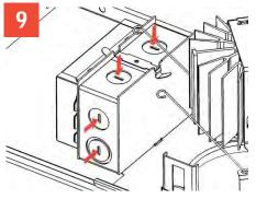
Remove knockouts on junction box to feed power supply to fixture. Supply wire must meet applicable electrical codes and be rated for a minimum of 90°C. Junction box is thru-wire rated for 8-No. 12 AWG conductors (4in-4out).
