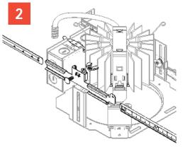
Assemble the channel bars to each side of the of the mounting frame with the included hardware. Leave the hardware loose to adjust the position of the frame in the ceiling.
