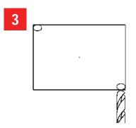
Drill a small hole at two corners of the sketched template.
