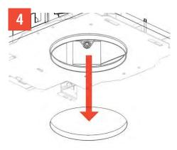
Position mounting frame through opening in ceiling.
