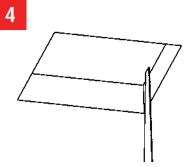
Using a keyhole saw, cut on sketched line. Return to section C-2 to complete the installation.
