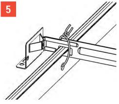
Secure channel bars to T-bar by means of wire ties.
