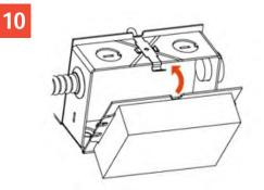
Complete necessary splices. Snap the door/driver assembly onto the junction box.
