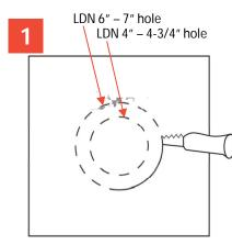
Cut ceiling opening slightly larger than the outside diameter on the mounting frame. 4" Ceiling opening: 4-3/4" (12.1cm). 6" Ceiling opening: 7" (17.8cm)
