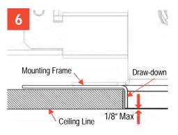
Adjust the mounting frame vertically to align the bottom edge of the draw-down to either flush or slightly above (1/8" max) the ceiling line.
