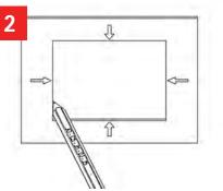
Using the square template, sketch the hole on the ceiling.
