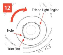
Align the opening in the trim with the tabs on the light engine. Rotate the trim clockwise until trim slot aligns with the hole in the trim holder. Secure trim with provided screw. Push the light engine up so it flush with the ceiling.
