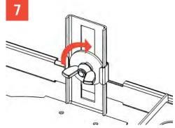
Re-tighten both vertical adjustment nuts.
