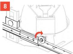
Re-tighten both channel bar clamping screws.
