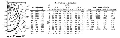
2BLT4 48L ADP LP835, 4960 delivered lumens, test no. ISF 36900P117, tested in accordance to IESNA LM-79
