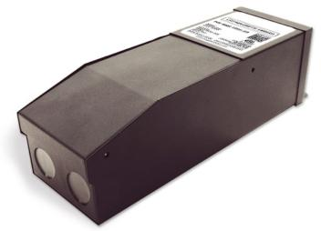
KLUS - MD-200-24 is the most compact LED driver on the market with a magnetic transformer core. It is equipped with two push-to-reset circuit breakers on the input and output, which protect both the load and driver. The driver is encased in a coated metal box that includes 2 knock-outs on the bottom to enable easy installation that complies with electrical code requirements.
