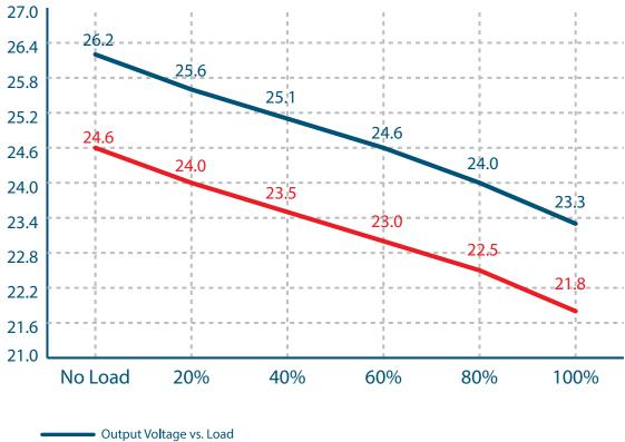
Output Voltage With a Typical Dimmer
