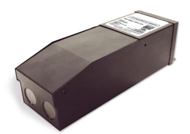
KLUS - MD-150-24 is the most compact LED driver on the market with a magnetic transformer core. It is equipped with two auto-reset breakers, one on the input and one on the output, which protect both the load and driver. The driver is encased in a coated metal. box that includes 2 knock-outs, one on each side, to enable easy installation that complies with electrical code requirements.
