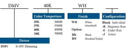
\*Field installed-Dimming Wire
