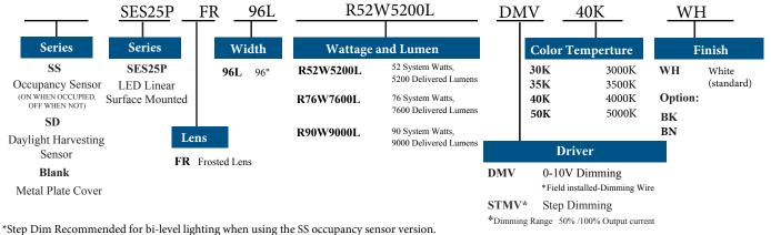
Step Diff Recommended for bi-level lighting when using the 55 occupancy sensor
