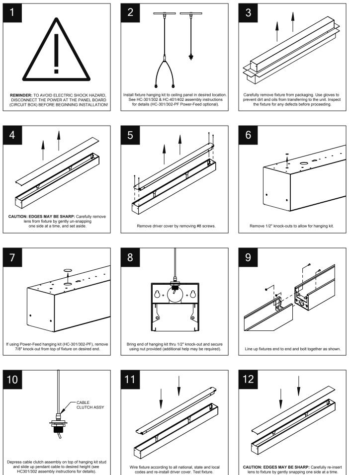
CAUTION: EDGES MAY BE SHARP: Carefully re-insert lens to fixture by gently snapping one side at a time.
