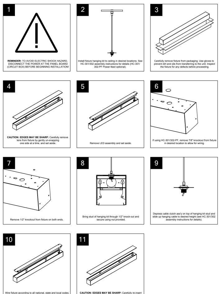
lens by gently snapping in one side at a time.
