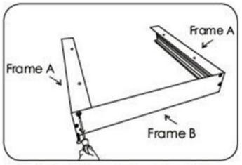
b, Fix the two "A" frames together with one "B" frame
