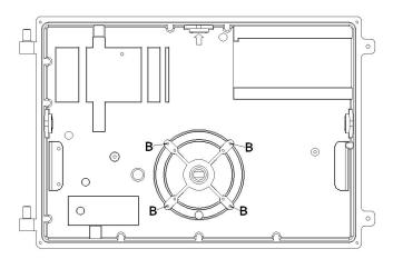
Method 2: Drill holes at the required three mounting points, mount the fixture by securing mounting screws (not provided) through the drilled holes, and seal the screw heads with appropriate waterproofing material. Then connect the input wires.
