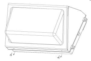
Step 4: Close the diffuser door and lock it with the 2 diffuser door screws.
