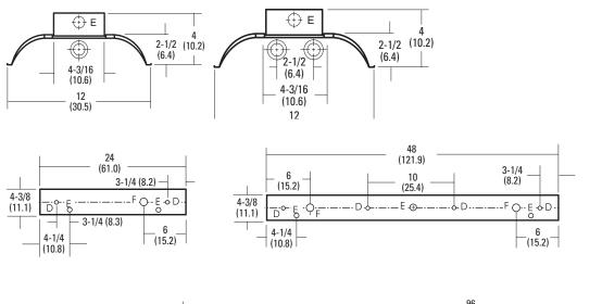
$$\begin{split} D &= 11/16 \; (1.7) \; \text{Dia.K.O.} \\ E &= 7/8 \; (2.2) \; \text{Dia.K.O.} \\ F &= 1-1/8 \; (2.9) \; \text{Dia.K.O.} \\ H &= 2 \; (5.1) \; \text{Dia.K.O.} \end{split}$$
