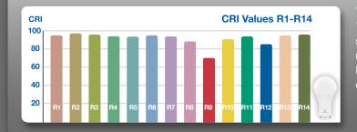
THE CRISP SERIES A19 9W GU24 lamp features a typical CRI 92, R9 70 and R13 95, providing crisp and vibrant colors across the whole spectrum. Its exceptional R9-R14 values (R9 & R13) provide redder reds, natural looking skin tones and whiter whites. In addition, this lamp's color temperatures fall within a 4-step Macadam ellipse to ensure minimal color deviation across lamps.
