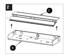
3. Determine appropriate knockout for removal in relationship to incoming power supply. To remove knockout, place standard screwdriver on edge of circle opposite retaining tab and gently strike with hammer until it releases. Grip edge with pliers and flex back and forth till knockout is removed.
