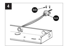
5. Position channel body (B) in desired mounting location and mark center point in small location of keyhole slot. Drill pilot hole at market locations. Screw in mounting screws (BB) leaving space for channel body. Slide channel (B) over mounting screws. Lift and shift channel into position and tighten screws.
