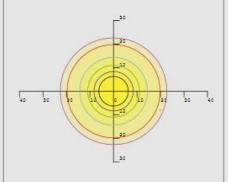
Mounting Height 10m, 0 Tilt, 20LUX-0.2LUX
