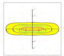
Mounting Height 10m, 0 Tilt, 50LUX-5LUX
