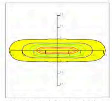
Mounting Height 10m, 0 Tilt, 50LUX-5LUX
