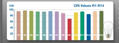
THE CRISP SERIES A19 9W lamp features a typical CRI 92, R9 70 and R13 95, providing crisp and vibrant colors across the whole spectrum. Its exceptional R9-R14 values (R9 & R13) provide redder reds, natural looking skin tones and whiter whites. In addition, this lamp's color temperatures fall within a 4-step Macadam ellipse to ensure minimal color deviation across lamps.
