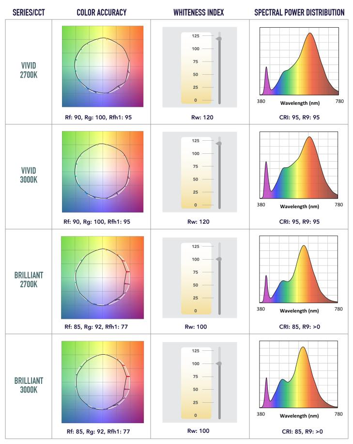
Rf: TM-30 metric measuring color fidelity (whether colors are similar to those under natural light). Rf is a more accurate version of the CRI Ra. Rf is 100 for natural light. Rg: TM-30 metric measuring color gamut (whether colors are more saturated than under natural light). Rg is 100 for natural light.
