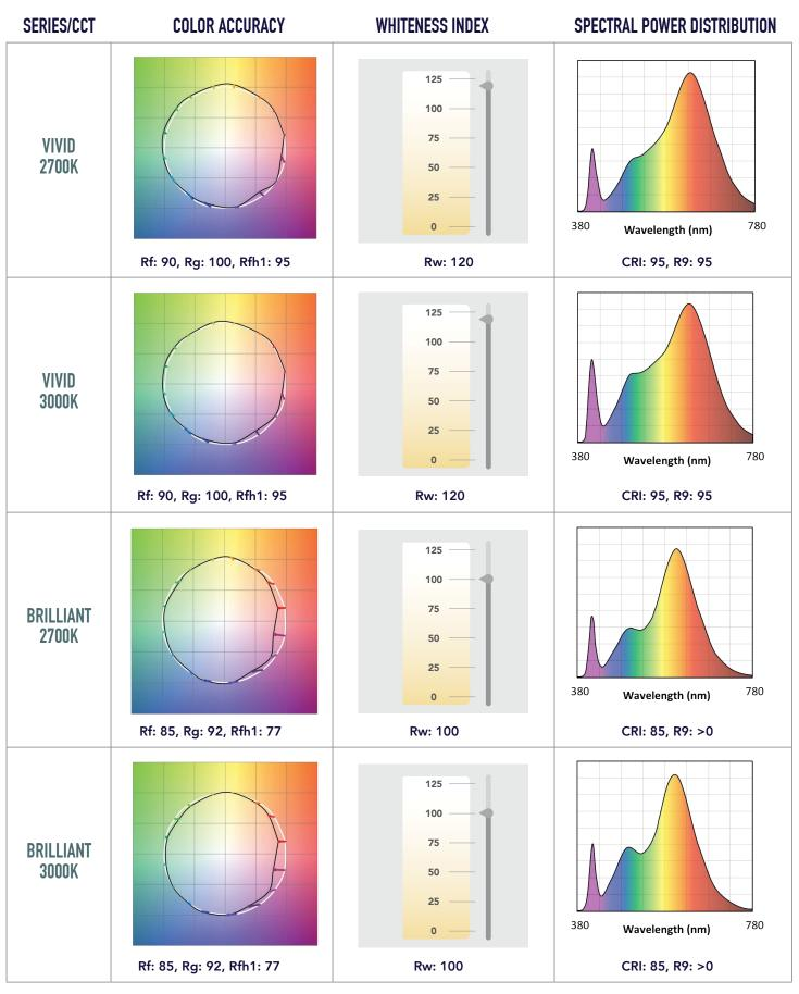
Rf: TM-30 metric measuring color fidelity (whether colors are similar to those under natural light). Rf is a more accurate version of the CRI Ra. Rf is 100 for natural light. Rg: TM-30 metric measuring color gamut (whether colors are more saturated than under natural light). Rg is 100 for natural light. Rfh1: TM-30 metric measuring color fidelity for red tones. Rfh1 is a more accurate version of the CRI R9. Rfh1 is 100 for natural light.
