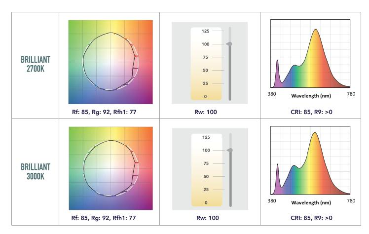
Rf: TM-30 metric measuring color fidelity (whether colors are similar to those under natural light). Rf is a more accurate version of the CRI Ra. Rf is 100 for natural light. Rg: TM-30 metric measuring color gamut (whether colors are more saturated than under natural light). Rg is 100 for natural light. Rfh1: TM-30 metric measuring color fidelity for red tones. Rfh1 is a more accurate version of the CRI R9. Rfh1 is 100 for natural light.
