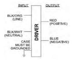
Input and output use lead-wires.
