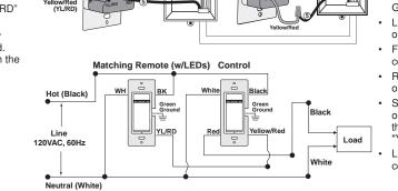
4-Way Wiring with Matching Remote (w/LEDs) Application
