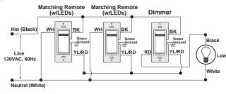
NOTE: The dimmer must be installed in a wall box that has a Load connection. The matching remote **must** be installed in a wall box with a Line Hot connection and a Neutral connection. A Neutral wire to the matching remote needs to be added as shown.
