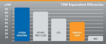
At 96 LPW, this lamp's efficacy is 15% higher than the Tier 1 LED A19 75W replacement industry average and exceeds new ENERGY STAR requirements by upwards of 70%. This energysaving performance makes this lamp a smart retrofit choice for incandescent and CFL bulbs.
