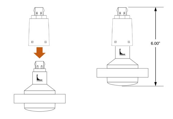
The extended CFL LED G24q Type B lamp will be approximately 6-inches in overall length (compared to 3.83" for just the lamp).
