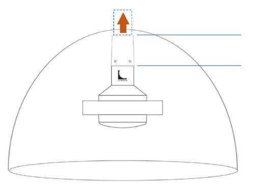
The extended CFL LED G24q Type B lamp will be approximately 2.25 inches closer to the fixture opening.
