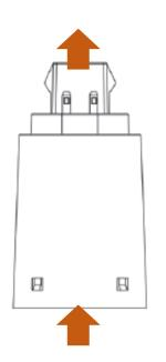
The other end of the accessory is a female G24q 4-pin socket into which the Lunera CFL LED G24q Type B lamp is installed.
