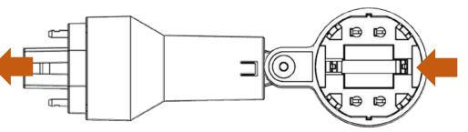
The other end of the accessory is a female G24q 4-pin socket into which the Lunera CFL LED G24q Type B lamp is installed.
