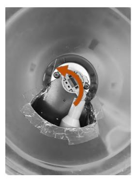
The swivel head is used to center the male G24q socket extender in the fixture.
