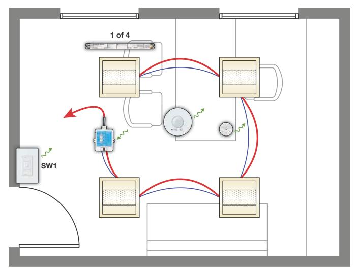
Line voltage wiringLow voltage wiring
