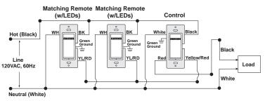
NOTE: The control must be installed in a wall box that has a Load connection. The matching remote must be installed in a wall box with a Line Hot connection and a Neutral connection. A Neutral wire to the matching remote needs to be added as shown.
