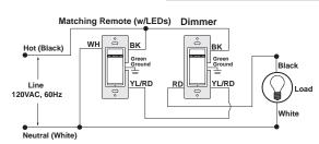
NOTE: The dimmer must be installed in a wall box that has a Load connection. The matching remote must be installed in a wall box with a Line Hot connection and a Neutral connection. A Neutral wire to the matching remote needs to be added as shown
