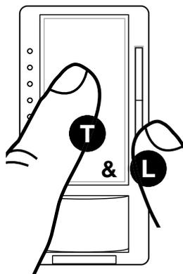
2. Adjust light output using **Raise/Lower** button until stable and not flickering. **Press and release the Tap** button to save setting.
