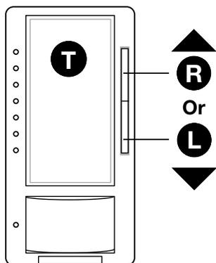
3. **Press and release Tap** button to turn load OFF, then press **Raise** button once. If load does not turn ON or remains unstable repeat and in **Step 2** increase light with **Raise** button.
