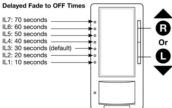
3. **To Save** the desired Delayed Fade to OFF, **Press the Tap** button. This will exit out of the Delayed Fade to OFF option and return to APM main menu.
