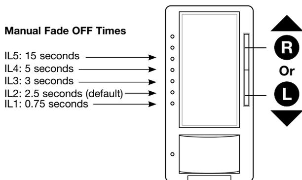
3. **To Save** the desired Manual Fade OFF Time, **Press the Tap** button. This will exit out of the Manual Fade OFF Time Option and return to APM main menu.
