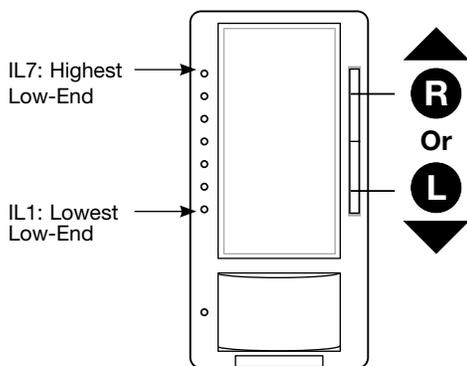
3. **To Save** the desired Low-End Trim setting, **Press the Tap** button. This will exit out of the Low-End Trim option and return to APM main menu.
