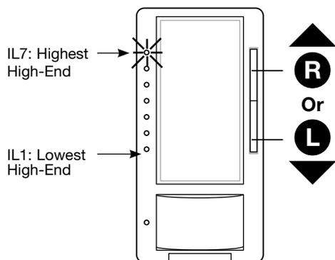
3. To save the desired High-End Trim setting, **Press the Tap** button. This will exit out of the High-End Trim option and return to APM main menu.
