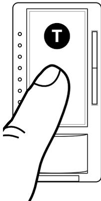
The default light setting has now been redefined. A single tap of the Tap button (when in Normal Operation, not APM) will now always return the dimmer to this selected light setting until preset is deactivated or reset. A double tap will always bring the lights to full intensity.
