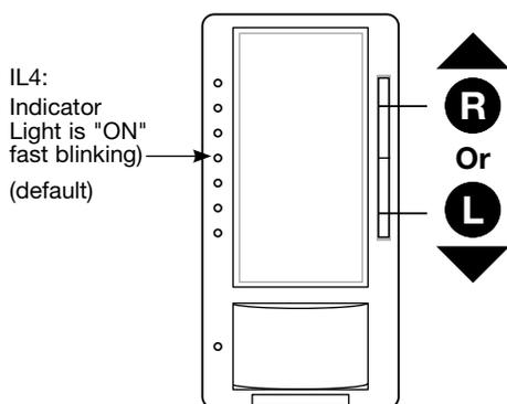
3. **To Save** the desired Enable/Disable Indicator Lights setting, **Press the Tap** button. This will exit out of the Enable/Disable Indicator Lights option and return to APM main menu.
