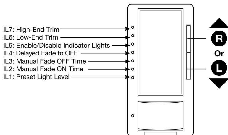
2. **To Enter** the desired option, **Press the Tap** button. Proceed to the specific Programming Option page to view programming instructions for desired Option.
