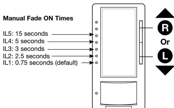
3. **To Save** the desired Manual Fade ON Time, **Press the Tap** button. This will exit out of the Manual Fade ON Time Option and return APM main menu.
